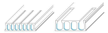
Fig. 2.14 The open cores at the ends of hollow core slabs
