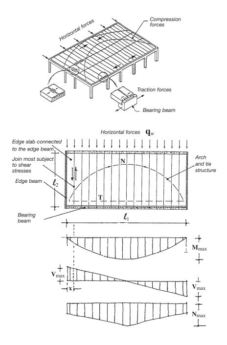
*Fig. 5.13 A diaphragm behaviour of the hollow core floor with an illustration of verification methods*
