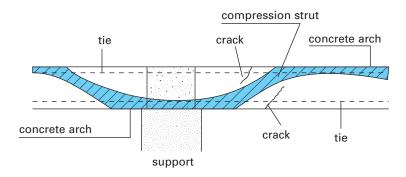
Fig. 4.10 The arch-tie mechanisms created in correspondence to supports of hollow core floor made continuous (Prof. Franco Levi - Politecnico of Turin 1983).
