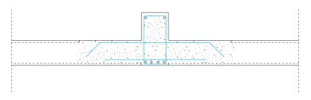
Fig. 4.29 Clear span floor suspended from a raised beam.
