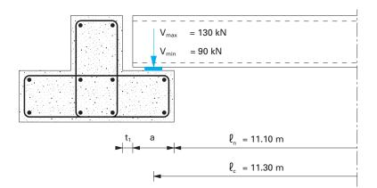
Fig. 3.18 Nominal length "a" of support of a hollow core floor on a precast inverted "T" beam
