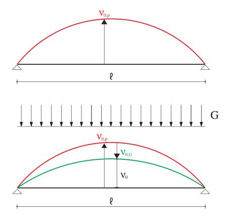
Fig. 5.17 Initial camber  $v_0$  on removal from casting bed
