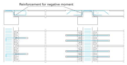
*Fig. 4.18 Hollow core floor in continuity on an inverted T beam.*
