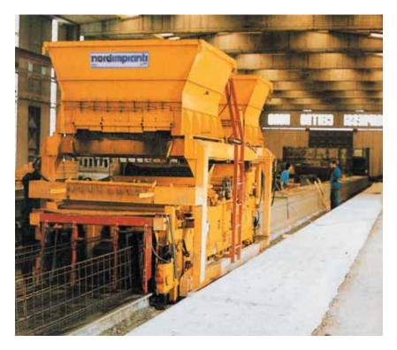
*Fig. 2.1 Slide-mould machine (slipform procedure)*
