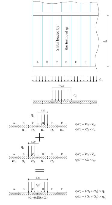
Fig. 5.21 Test overload  $q_c$  and in-service load  $q_s$ Calculation of elastic sag for the final inspection test of a hollow core floor.
