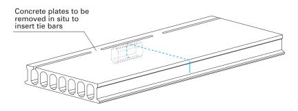
Fig. 4.5 Slab prepared to house perimetric tie bars. The transverse bars anchored in the hollow core slab that restrain the floor to the perimetric tie in seismic zones shall be at least two for a floor span of l > 6.0 m and at least one for spans of 4.0 < l < 6.0 m and shall have area of at least 33.3 mm<sup>2</sup>/m (Italian Prefab Regulations 2.11.2. e).
