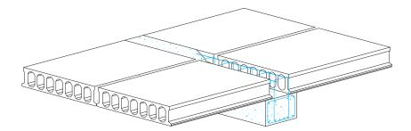
*Fig. 4.26 Beam previously cast in situ to be self-supporting of the dead weight of the floor itself and the finishing casting.*
