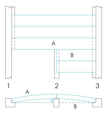
Fig. 5.15 To avoid ugly differences in flatness between adjacent slabs A and B, it is necessary to superelevate the intermediate support
