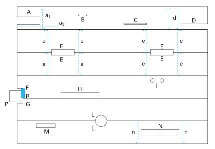
Fig. 2.18 Several possibilities of cut-outs and holes that can be made in 120 cm-wide hollow core slabs using the proper techniques
