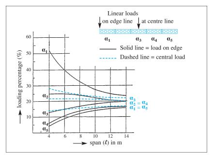
Fig. 5.4 Transverse distribution factors for linear loads
