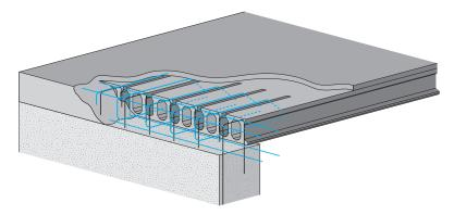
*Fig. 4.40 Connection between hollow core floor and retaining wall, with fixed end.*
