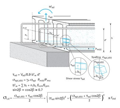
Fig 4.34 Principal stress  $\sigma_{ld}$ , that is, the combination of spalling stress with suspension stress in the end of web "i" of the hollow core slab when the ordinary support is lacking.
