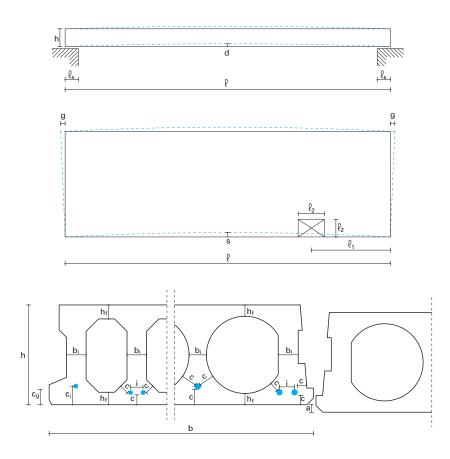
Fig. 2.23 Geometric references for dimensional and assembly tolerances
