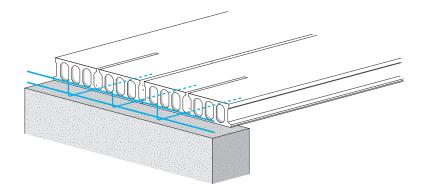
Fig. 3.19 The reinforcement at the supports of the hollow core floor as for Art. 7.0.a of Italian Standard
