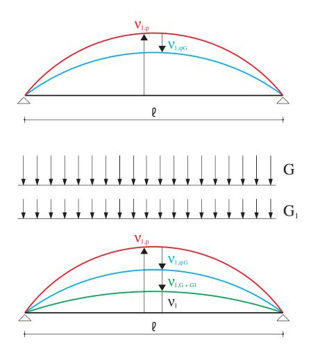
*Fig.* 5.18 *Camber after installation*  $v_1$  *at time*  $t_1$ .
