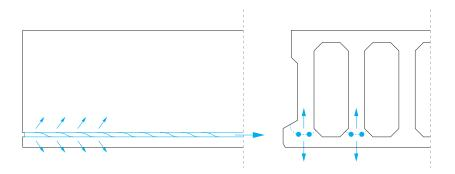
*Fig. 3.10* Splitting at the slab end may cause a small crack that unites strands that are too close together.
