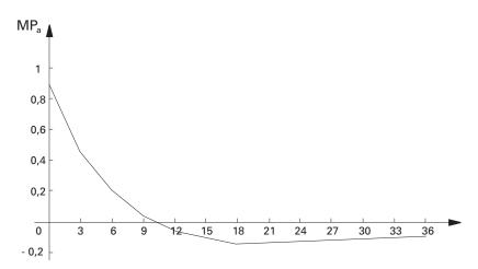
Fig.3.15 Trend of spalling tensile stress in the longitudinal sense at halfheight of the web (FIP Recommendations Precast Prestressed Hollow Core Floors 2.2.1)
