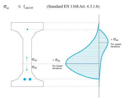
Fig. 3.14 Representation of spalling intensity  $\sigma_{sp}$  generated by the lower tendons and the upper tendon in a web of the hollow core slab.
