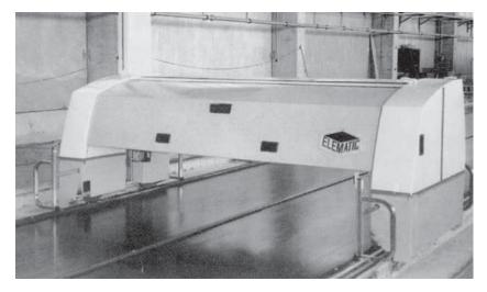
*Fig. 2.13 CAM plotter machine equipped with an automatic marking device.*
