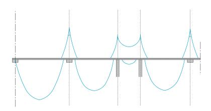
Fig. 4.12 Trend of the maximum negative and positive moments in a continuous floor due only to permanent and occasional loads in the  $2^{nd}$  phase:
