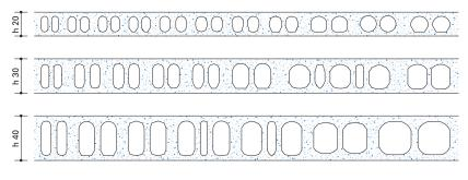
Fig. 2.8 Types of voids in hollow core slabs
