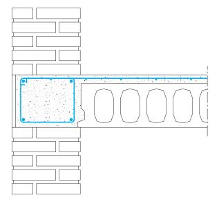
*Fig. 4.3 Lateral connection with a resistance-welded mesh inside the concrete topping.*
