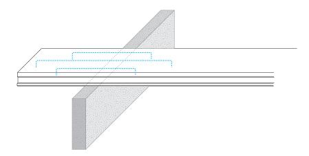
Fig. 2.16 Example of longitudinal reinforcement inserted manually in the still-fresh hollow core slab in correspondence to a support with a heavily loaded cantilever
