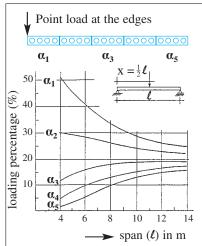
Fig. 5.6. Transverse distribution factors of point loads "at the edges"
