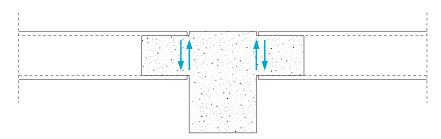
Fig. 4.32 Shear stresses in the attachment section of concrete nuclei to the beam when shear reinforcement is missing.
