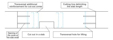
Fig. 2.12 Manual operations on a slab immediately after casting.
