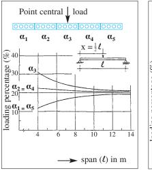
Fig. 5.5. Transverse distribution factors of point loads "at central line"
