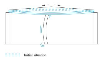
Fig. 5.16 The slopes of the cover must be assured even after the deformations at infinite time. The latter may even compromise the stability of partition walls.
