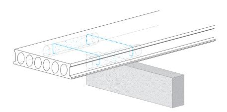
Fig. 2.15 Example of transverse reinforcement inserted manually into fresh concrete of a partially supported slab.
