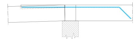
*Fig. 4.11* Lacking terminal anchorage at the lower edge, the stressed steel may cause the problem seen here.
