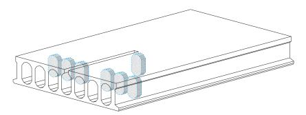
*Fig. 4.15 Slab end prepared for casting of a small flange corroborant with the bearing beam.*
