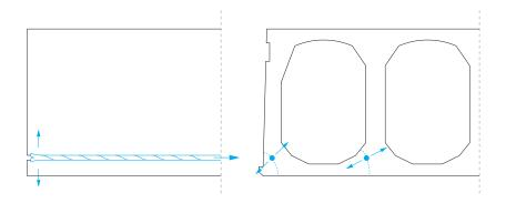
Fig. 3.9 Bursting may cause small cracks to appear in the hollow core slab end
