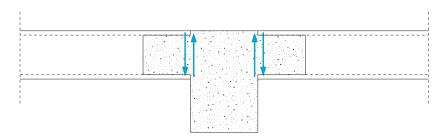
Fig. 4.33 If the ends of the hollow core slab are rough, shear stresses at the interface with the beam are distributed throughout the entire end section of the slab.
