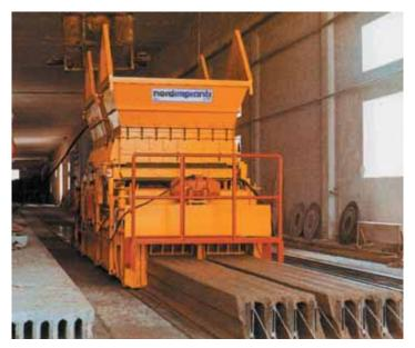
Fig. 2.4 Continuous casting of concrete
