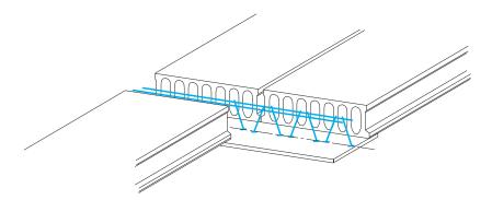
Fig. 4.24 The hollow core floor supported by a reticular steel beam.
