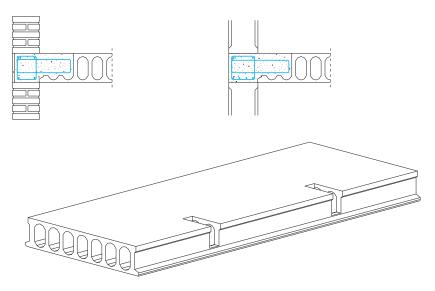
Fig. 4.2 Lateral cuts in a slab without topping for hooking bar housing
