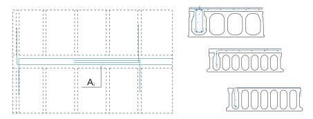
*Fig. 4.4 Edge tie bars incorporated in the hollow core slab or in the final longitudinal join in presence and absence of concrete topping.*
