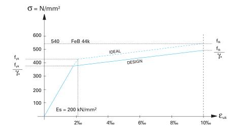
*Fig. 5.2 Design stress-elongation diagram for normal reinforcement steel*
