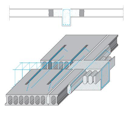
Fig. 4.27 The beam-floor connection with a clear span
