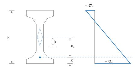
*Fig. 3.7* The inertial core and the eccentricity of a prestressing tendon
