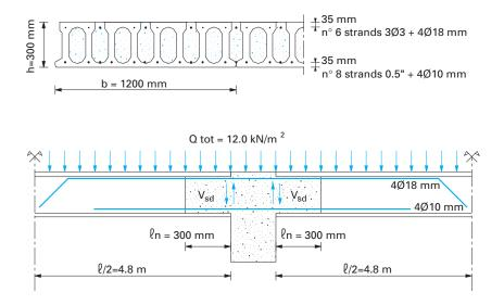
Fig. 5.20 Calculation of deformations of a hollow core floor with h = 300 mm
