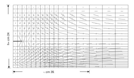
Fig. 3.13 Principal stresses at the end of a prestressed hollow core slab having depth 24 cm and tendons 3 φ 3 mm.
