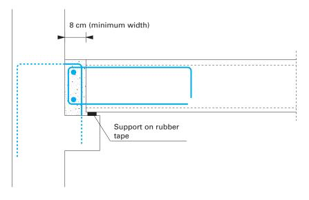
*Fig. 4.41* The wall - hollow core floor connection with a bond of simple support.
