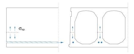
Fig. 3.11 Spalling may cause lesions in the prestressed slab end
