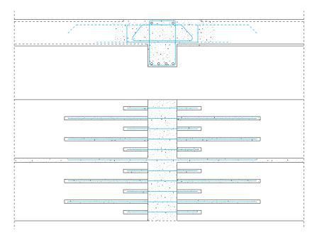
*Fig. 4.28* An example of stirruping of the in situ cast nuclei in the cores and in the longitudinal union.
