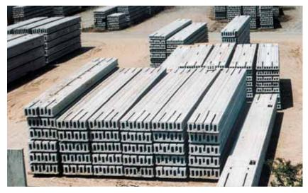
Fig. 2.6 Hollow core slab storage yard
