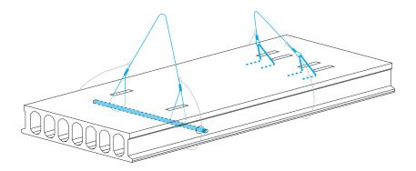
Fig. 2.19 Holes for lifting with cables and blocking rod, or with tested and certified steel forks. Note the safety cables to be detached just before placing the slabs in position
