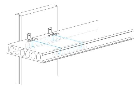
*Fig. 2.17 Example of the proper anchoring of boltable profiles on the outer edge of a hollow core slab.*
