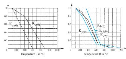
Fig. 5.9. Variation in the characteristic strength of concrete with variations in temperature
