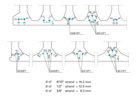
Fig. 2.11 Correctly placed reinforcement. Having assured control of production, the minimum design values for a single strand indicated above for "c" admit the maximum negative tolerance of – 5 mm (EN 1168 par. 4.3.3.1 and ENV 1992-1-1 par. 4.1.3.3. Point 8).
