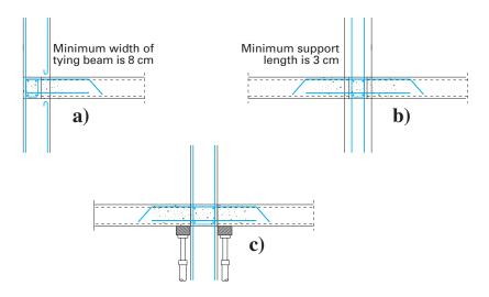
*Fig. 4.39* The connection between hollow core floor and reinforced concrete parting wall.
