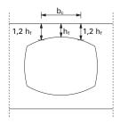
Generally speaking, the thickness of the vertical webs between voids is never less than  $30 \div 35$  mm and it increases in slabs of greater depth or more subject to shear stress.
