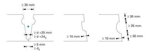
Fig. 3.5 Longitudinal join: shapes and minimum dimensions (proposed in the European Standard EN 1168 Art. 4.3.1.4 and Informative Annex B)
