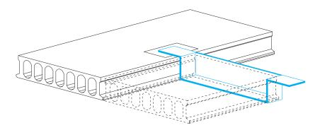
*Fig. 4.43 Example of a small steel beam having a span of 120 - 240 cm to support hollow core slabs in the presence of large openings.*
