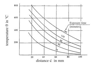
Fig. 5.11 Mean temperature values in the webs of hollow core slabs  $h = 200 \div 400 \text{ mm}$  as a function of distance from the intrados
