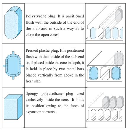
Fig. 2.21 Plugs for hollow cores.
