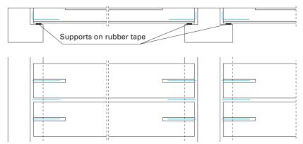
*Fig. 4.17 Hollow core floor with simple support on inverted T and L beams.*
