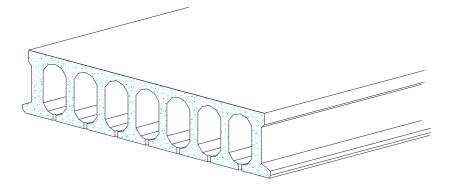
Fig. 2.20 Boring for the drainage of rainwater. Diameter about 6 - 8 mm
