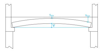
Fig. 5.14 The minimum height between floors must be measured at the supports of the hollow core floor.
