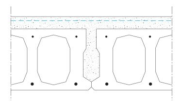
Fig. 3.3 Longitudinal join with reinforced or non-reinforced topping
