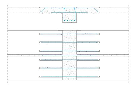
Fig. 4.31 Continuity reinforcing bars are provided with a distance between centres which on the average is not more than 30 - 40 cm.
