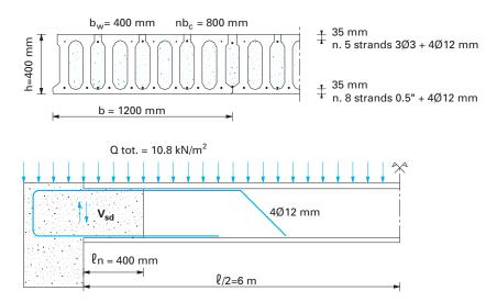
Fig. 4.37 Slipformed hollow core slab h = 40 cm, reinforced with eight 0.5" strands.
