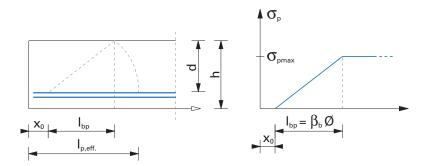
Fig. 3.20 The transfer of prestressing in hollow core slabs
