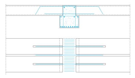
*Fig. 4.25 The floor-beam connection cast in situ with length of support of the floor.*
