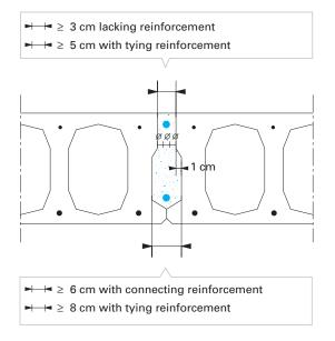
Fig. 3.4 Longitudinal join: minimum dimensions in presence of connecting reinforcement and when tying reinforcement is called for (Italian Prefab Regulations, par. 2.11.2 b point 3)
