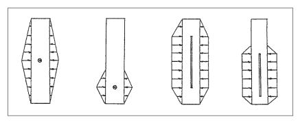
Fig. 5.7. Distribution of shear forces in the longitudinal join
