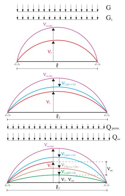
Fig. 5.19 Deformation at infinite time  $v_{\infty}$  of a hollow core floor of span  $\boldsymbol{\ell}$ , compared to the initial camber  $v_1$  once installed, in presence of all permanent and long-term variable loads (quasi - permanent load condition), with the real conditions of restraint in service and the corresponding calculated span  $\boldsymbol{\ell}_2$ .
