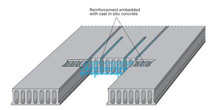
*Fig. 4.44 Example of a reinforced concrete beam cast in situ to support hollow core slabs involved in a large opening.*
