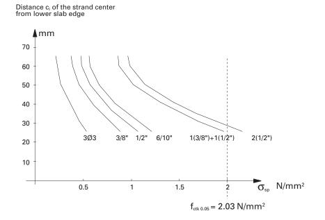
Fig. 3.16 Values  $\sigma_{sp}$  for each cross section of hollow core slab can be supplied by each producer already in table form for the different types of strand.
