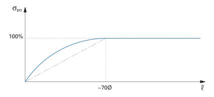
*Fig. 3.8 Development of prestressing in the anchorage zone*
