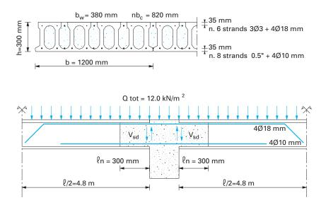
Fig. 4.35 Verification of a slip-formed hollow core floor of depth h = 300 mm as a clear span between beams cast in situ (floor without direct support on the beam).
