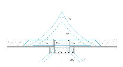
Fig. 4.13 Negative moment  $M_i$  decreases to  $M'_i$  due to greater deformability, both elastic and viscous, of concrete with strength  $f'_{ck}$ . Consequently the positive moments of the span increase by the same amount.
