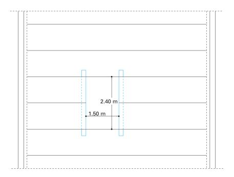
*Fig. 4.42 Example of a large hole in a hollow core floor.*
