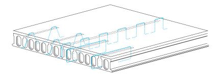
*Fig. 3.6 Possible connecting reinforcement between hollow core floor and the corroborant cast in situ topping*
