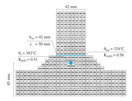
Fig. 5.8. Example of thermal mapping at 120 minutes of a hollow core slab h = 240 mm with strand 45 mm from the intrados and with 2% humidity
