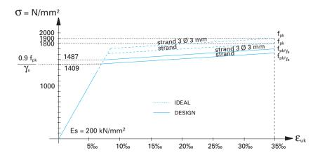
Fig. 5.2 Stress-elongation diagram of prestressing steel
